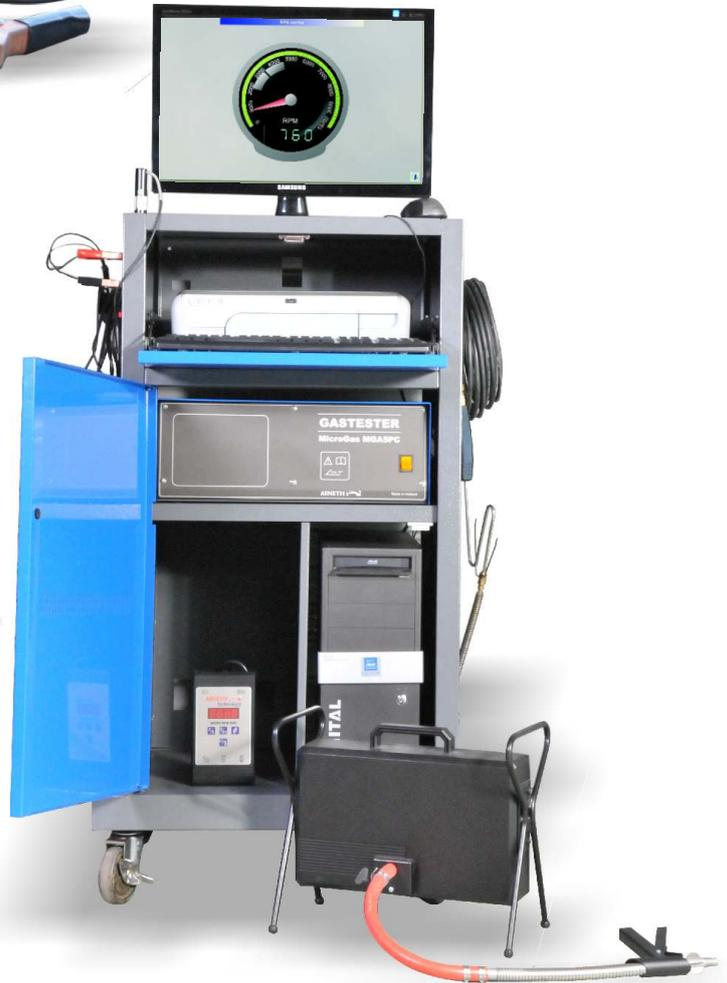
Complete Emission test station MCA-PC
